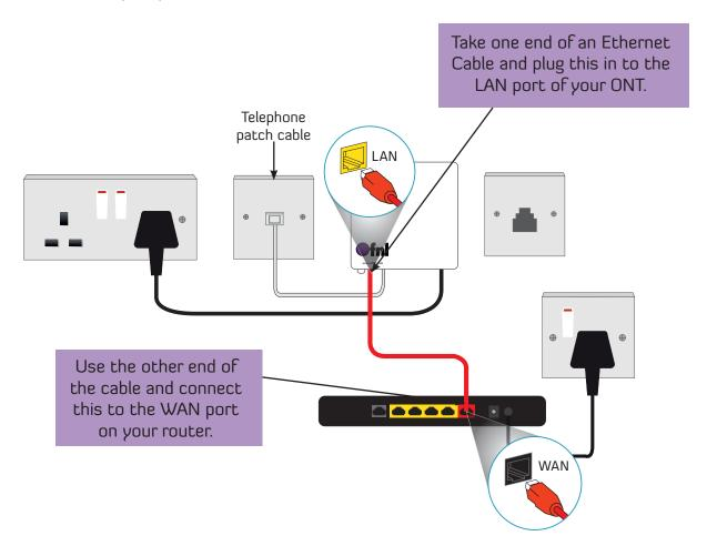
To connect your router to your internet enabled devices using a wired connection;
